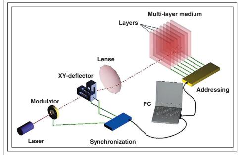
*Fig. 1:* This volumetric 3-D display system employs a multilayer FLC medium and optoelectronic addressing.
